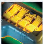
wind the wires around the probes and store away in the back storage housing. This helps extend probe life and keeps them ready for the next job.
